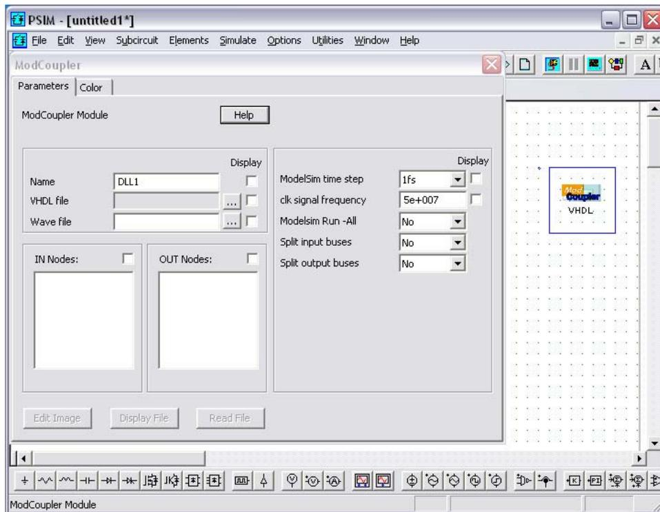
Fig. 3: ModCoupler-VHDL module dialogue window.
