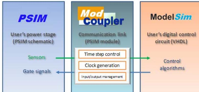
Fig. 1: Co-simulation architecture.
